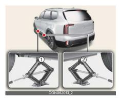
Insert the wheel lug nut wrench into the jack and turn it clockwise, raising the vehicle until the tire just clears the ground. This measurement is approximately 1 inch (30 mm).
