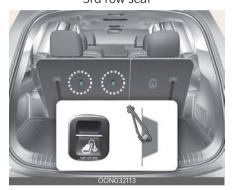
First secure the child restraint with the LATCH lower anchors or the seat belt. If the child restraint manufacturer recommends that the top tether strap be attached, attach and tighten the top tether strap anchor.
