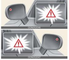
The warning light on the outside rear view mirror (side view mirror) and headup display (if equipped) will appear when the vehicle on both lanes is detected from the rear.
