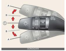
The ENGINE START/STOP button must be on for the turn signals to function. To turn on the turn signals:
