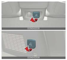
The AC inverter supplies 115 V / 150 W electric power to operate electric accessories or equipment.
