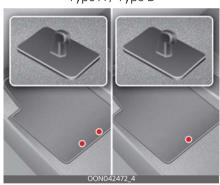
When using a floor mat on the front floor carpet, make sure it attaches to the floor mat anchor(s) in your vehicle. This keeps the floor mat from sliding forward.
