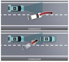
[A]: Your vehicle, [B]: Front vehicle If a vehicle cuts in front of your vehicle, Leading Departure Alert may not operate properly. When the vehicle ahead sharply steers
