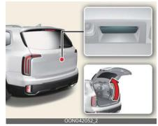
When the liftgate is closed, press the power liftgate open/close button to open the liftgate.
