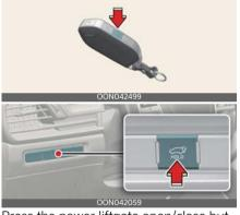
Press the power liftgate open/close button for 1 second. The liftgate opens or closes with a warning sound.
