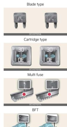
\* Left side: Normal, Right side: Blown This vehicle has 2 (or 3) fuse panels, one located in the driver's side panel bolster, the other in the engine compartment
