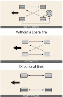
Rotate radial tires that have an asymmetric tread pattern only from front to rear and not from right to left.
