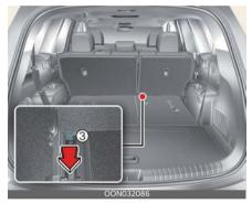
If the walk-in switch (1 or 2) in the 2nd row (in the upper part of the 2nd row seatback or the outer part of the seat) does not work, pull the strap (3) on the bottom left of the seat in the 2nd row. It works just like the walk-in switch and you can move the seat forward along with the seatback.
