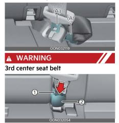
Do not separate the mini tongue (1) and mini buckle (2) even if there is not an occupant.
