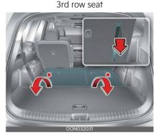
To use the rear seat, lift and pull the seatback backward. Pull the seatback firmly until it clicks into place. Make sure the seatback is locked in place. When you return the seatback to its upright position, always be sure it has locked into position by pushing on the top of the seatback.
