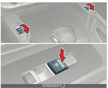
The temperature setting of the seat changes according to the levers/ switches position.
