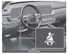
If you start to drive without the seat belt fastened or you unfasten the seat belt when you drive over 5 mph (9 km/h) and less than 12 mph (20 km/h), the corresponding warning light will appear. The
