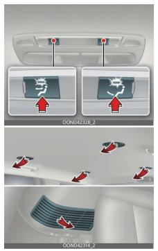
The rear mode is selected by pressing the rear mode selection button on the rear control panel as follows:
