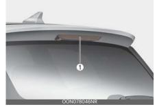
The LED lamps cannot be replaced as a single component because it is an integrated unit. The LED lamps have to be replaced with the unit.
