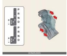
Press the brake pedal and the lock release button when shifting.
