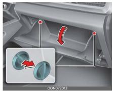
2. With the glove box open, pull the pin and the support strap (1).
