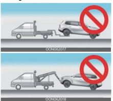
• Do not tow the vehicle backwards with the front wheels on the ground as this may cause damage to the transmission.
