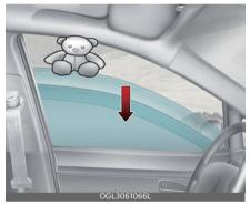
If the window detects the resistance while the power window switch is pulled up continuously, the window will stop upward movement then lower approximately 1.2 inches (3 cm).
