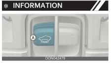
The sunshade opens automatically when the sunroof glass is opened by pushing the sunroof switch (A) rearward, but the sunshade does not close automatically when the sunroof glass is closed. Also, only the sunshade cannot be closed when the sunroof glass is opened.
