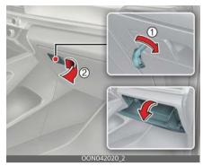
The glove box can be locked and unlocked with the mechanical key (1). To open:
