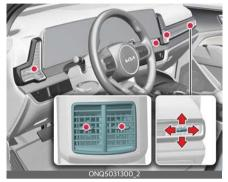
You can adjust the direction of air delivery from these vents using the vent control lever as shown.
