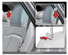
• To remove the headrest, raise it as far as it can go then press the release button (1) while pulling the headrest upward (2). • To reinstall the headrest, put the headrest poles (3) into the holes while pressing the release button (1).
