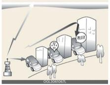
AM and FM radio signals are broadcast from transmitter towers located around your city. They are intercepted by the radio antenna on your vehicle. This signal is then processed by the radio and sent to your vehicle speakers.
