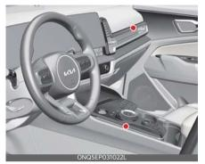
The ambient lights are applied to the front crash pad and the center console. When the headlamp light is on, the ambient light is on at the same time could be set in the infotainment menu. Refer to the infotainment manual for details.
