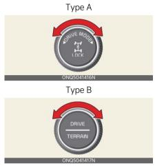
The Drive mode is activated by turning the knob.
