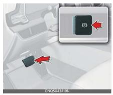
Releasing the parking brake with EPB switch,
