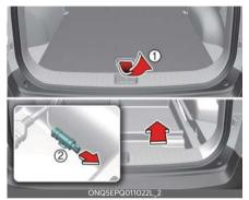
If the charging connector does not disconnect due to battery discharge and/or failure of the electric system, open the luggage board (1), remove the storage box and slightly pull the emergency cable (2). The charging connector will then disconnect.
