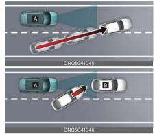
[A]: Your vehicle, [B]: Front vehicle If a vehicle cuts in front of your vehicle, Leading Departure Alert may not operate properly.
