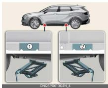
8. Insert the jack handle into the jack and turn it clockwise, raising the vehicle until the tire just clears the ground. This measurement is approximately 1.2 inches (30 mm). Before removing the wheel lug nuts, make sure the vehicle is stable and that there is no chance for movement or slippage.
