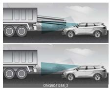
If the vehicle in front of you has cargo that extends beyond its bumper, or when the vehicle in front of you has an unusually high ground clearance, additional special attention is required. Forward Collision-Avoidance Assist may not be able to detect cargo extending from the vehicle. Maintain a safe braking distance from the rearmost object, by steering, slowing, and braking as needed.
