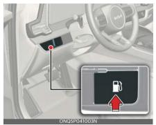
2. Wait until the fuel tank is depressurized. The message is displayed when the fuel filler door unlocks after the fuel tank is depressurized.
