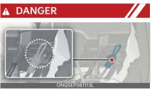
Pull or cut the service interlock connector to cut off the high voltage of the battery in an emergency. Service interlock connector cannot be reused when cut.
