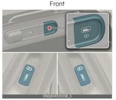
Plug the cable into the USB port, and charging will begin.
