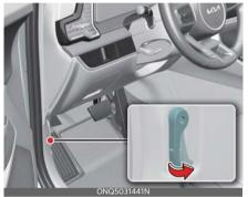
2. Go to the front of the vehicle, raise the hood slightly, push the secondary hood release lever (1) to the left and lift the hood (2).
