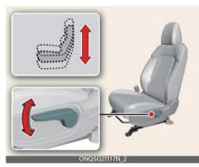
To change the height of the seat cushion, push the lever upwards or downwards.
