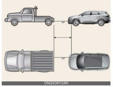
• Use a towing cable or chain less than 16 feet (5 m) long. Attach a white or red cloth (about 12 inches (30 cm) wide) in the middle of the cable or chain for easy visibility.
