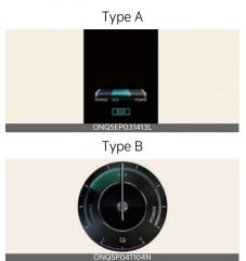
The hybrid system gauge indicates whether the current driving condition is fuel efficient or not.
