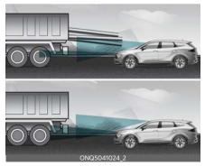
If the vehicle in front of you has cargo that extends beyond its bumper, or when the vehicle in front of you has an unusually high ground clearance,
